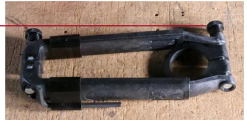
3. Disassemble the front end of the arms. This includes a washer, ring, and bolt.
