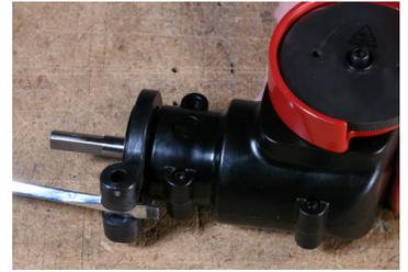
6. Once the ring is on the TSPC1, reassemble the front of the Rotary TurboShear® arms onto the ring. Slide the bolt through, add the washer, and tighten the thumb screw.
