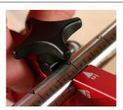
**5.** Slide bearing carrier to the correct bend depth and tighten thumbscrew when set.
