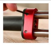
1. Loosen the set screw retaining shaft for the straight (non-angled) roller:
