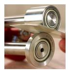
3. Insert material between rollers and rotate the shaft with 3 dots until the rollers on both shafts rotate when the material moves through the rollers.
