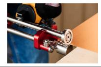
**2.** Glide the bender along the edge of the material, raising the handle slightly in the direction of the bend to initiate a bend line. The initial crease formed at this point is critical to set the course for the bender to follow.
