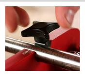
2. Loosen the thumb screw
