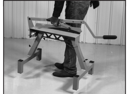
6. When transporting tool, replace cross pin to lock handle and blade in place.
