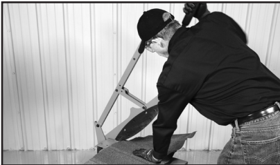
1. Remove cross pin that locks handle and blade assembly. Keep pin for future use.
