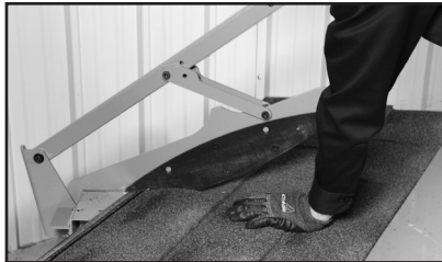
2. Lift handle to open tool throat.
